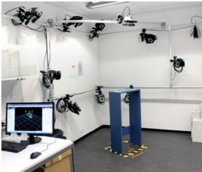
Figure 2: Motion analysis laboratory, equipped with a set of cameras to assess finger movements during daily activities.
