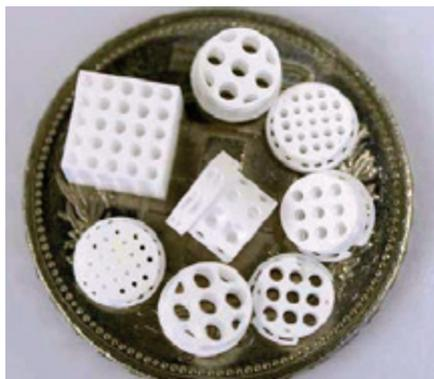
Figure 1 Diverse calcium phosphate-based bone substitutes produced by additive manufacturing (Ghayor & Weber FE (2018); *Frontiers in Physiology* doi: 10.3389/fphys.2018.00960)
